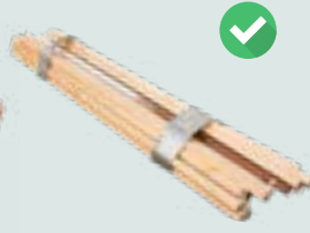
Timber – 12 pieces neatly stacked and no longer than 1.5 metres
