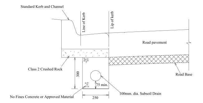
N.B. Inspection Openings at back of Kerb and Channel at 80m. spacings
