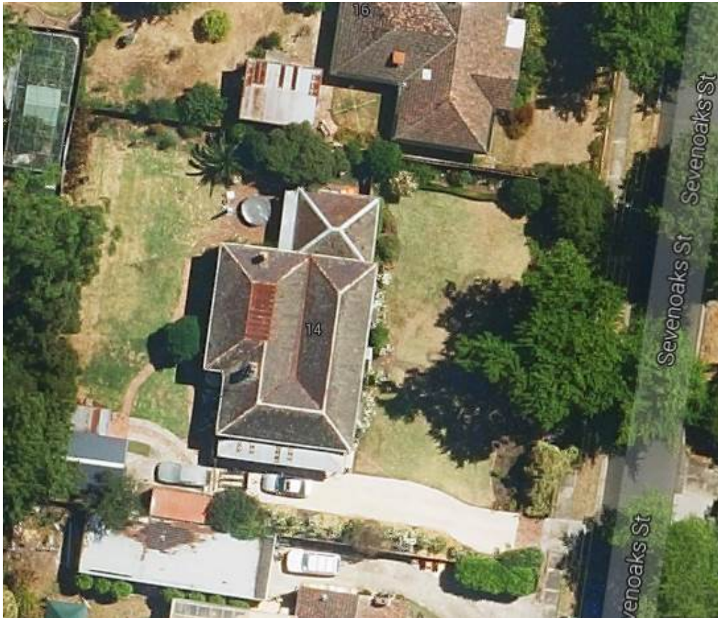
Figure 1. The former farmhouse on its reduced block. The former front elevation (at bottom) is indicated by the iron-roofed verandah. It originally wrapped around the west (left-hand) side as far as the chimney. The recent rear wing is visible at top. (Google Maps, accessed Dec. 2015)
