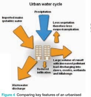
water cycle and an integrated water cycle (that incorporates water sensitive urban design) (Adapted from Hoban, 2006)
