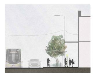
Figure 9 - Street section showing widened footpaths, safe cycle path, and additional tree planting (indicative diagram only).
