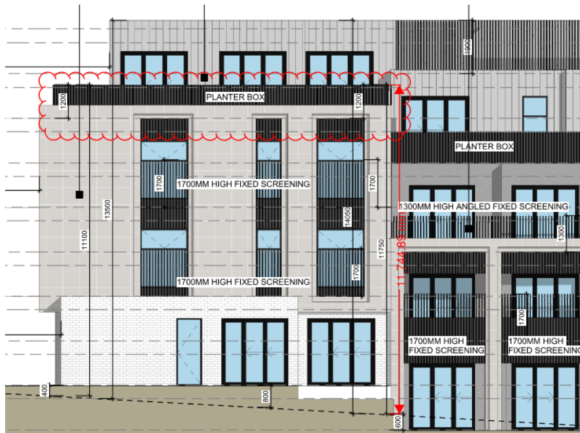
Figure 1 - Extent of non-compliance (clouded in red) to the western elevation at third floor level balcony
