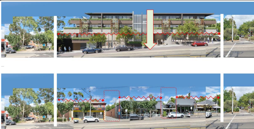
Figure 2: An extract of the existing (bottom) and proposed (top) street elevations demonstrating the difference between the existing and proposed street façades. Note how the accessway/lane and arcade break the continuity of the existing row of shops into three separate volumes. The extension of the central walkway to the street can help create a gap in the street façade, adding visual relief and reducing visual bulk.
