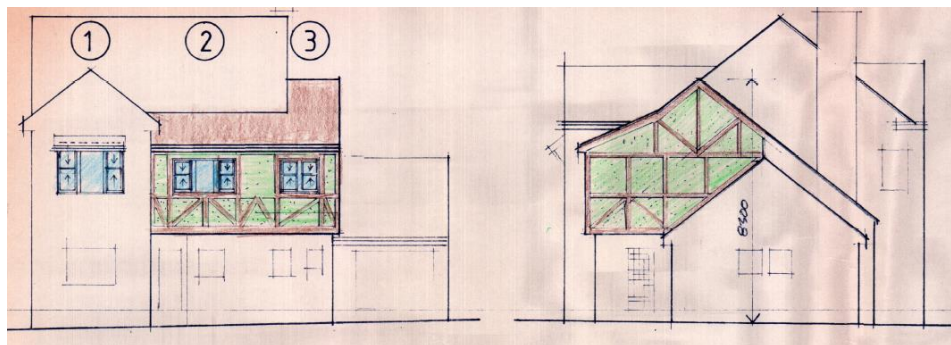
Figure 12. East and north elevations showing first floor addition made to the rear of the house by Melbourne Extensions and Designs, 1994 (City of Boroondara Building Plans 99329).
