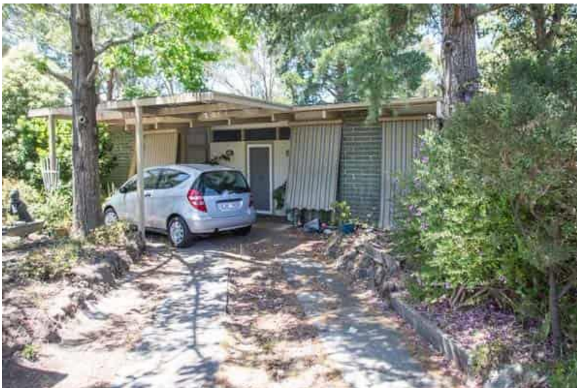
Figure 33 'Dome 32' One of the houses Knox designed for the Hillcrest Estate with non-load bearing internal stud walls, a Stramit ceiling and a malthoid and gravel roof (usually replaced). Photo: Tony Knox Source: AlistairKnox.org https://alistairknox.org/akimages/636
