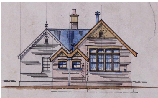
Figure 5. Front (east) elevation drawn for the 1907 additions. The new parts are shaded pale pink. (Source: PROV VPRS3686/P7/958)
