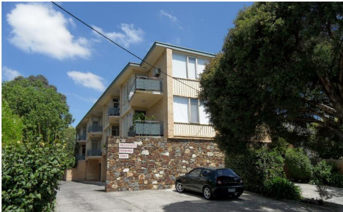
Figure 6. View of the principal elevations of the building (facing south-west from Denmark Hill Road). Note the cantilevered massing of the upper floors above the feature stone wall. The splayed balconies run the depth of the east elevation. The wall-mounted air conditioning unit visible at second-floor level is a later addition. (Source: Trethowan Architecture, 2017)
