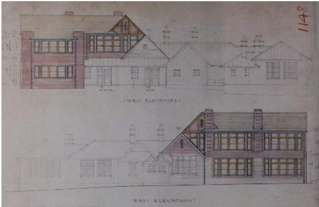
Figure 11. West (rear) and east (front) elevations drawn for the 1946-47 additions. Coloured sections indicate the proposed additions and changes to the building. (PROV VPRS 3686/P7/960)
