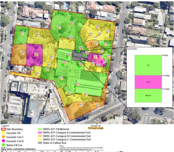
Soil classification identified in the Soil Contamination Management Plan
